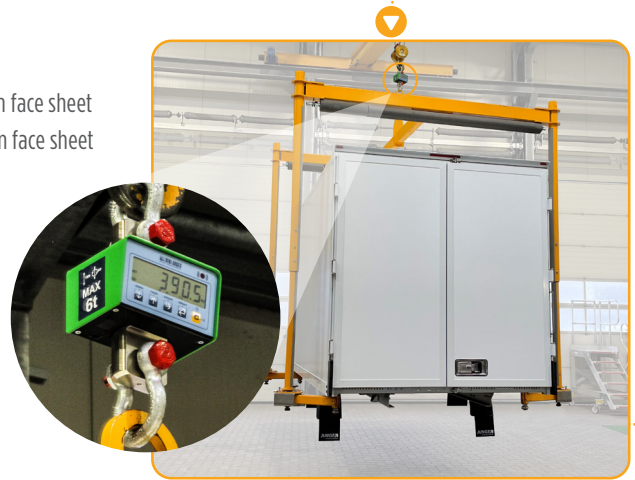
Unladen weight of body (length 4400 mm) incl. substructure and rear doors
